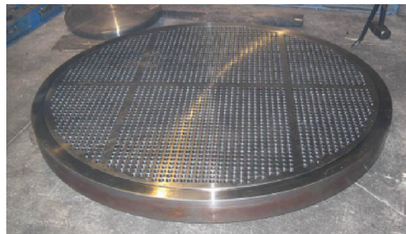
↑ Heat Exchanger End Plate
